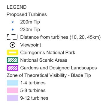
This drawing is based upon computer generated Zone of Theoretical Visibility (ZTV) studies produced using the Viewshed routine in the Visibility Analysis plugin for QGIS.
